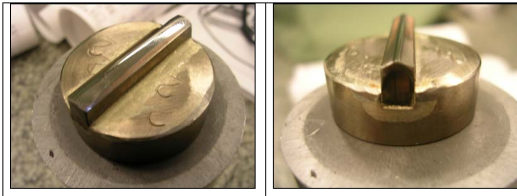
Figure 4. The forging tool tips used in ultra burnishing.
